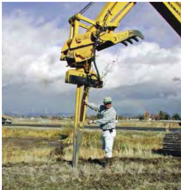
Figure 25: The use of a stinger for vegetative plantings (courtesy nativerevegetation.org).
