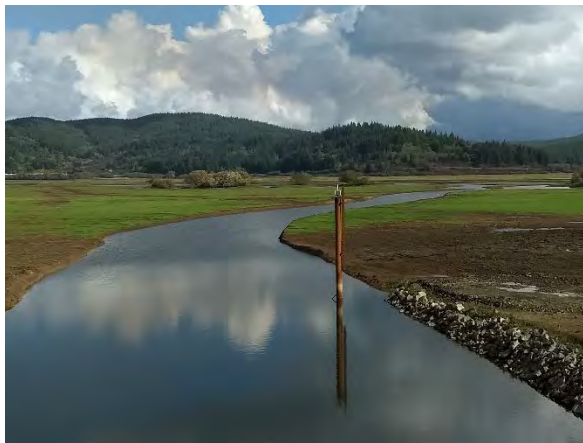
Figure 6. Permanent steel stilling wells house water level loggers maintained by Northwest Hydraulic Consulting (NHC), left. Data is transmitted via RTU to the network computer on-site every 15 minutes.
