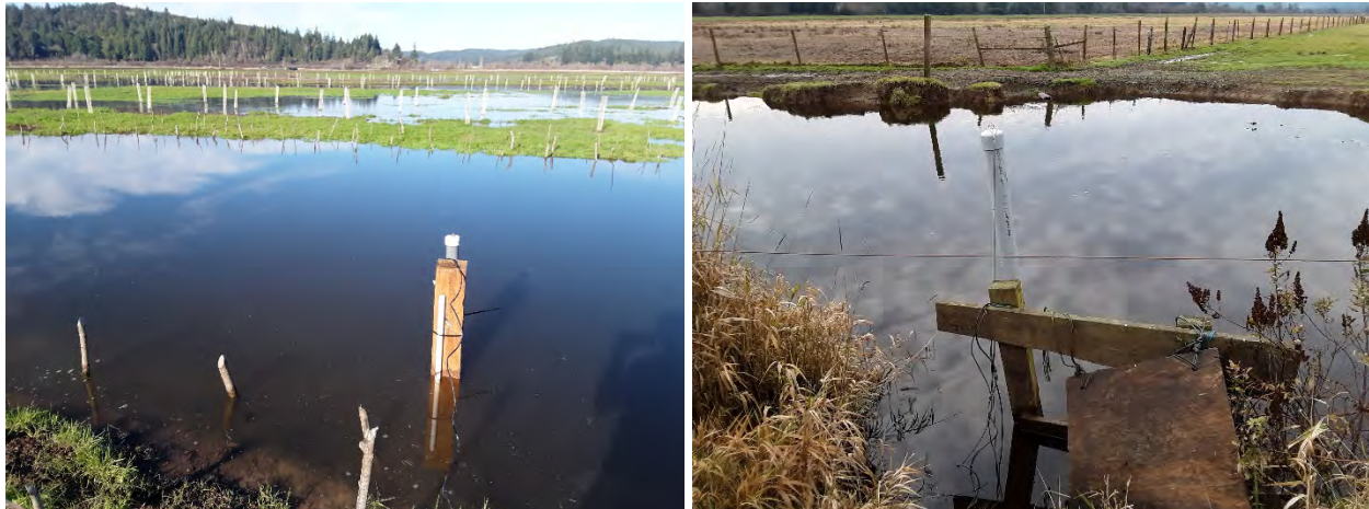
Figure 5. Permanent wooden posts with PVC stilling wells attached to house water level loggers within (left) and hang DO loggers from the cap (right). Temperature is collected by both water level and DO loggers.
