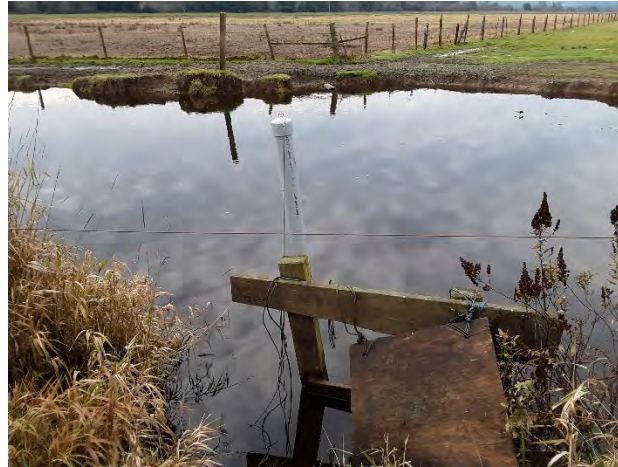
Figure 24. The stilling well at dissolved oxygen monitoring location WL22. The logger is hung off the cap of the stilling well to allow for better flow around the optical sensor.
