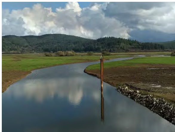
Figure 19. Permanent wooden posts with PVC stilling wells attached to house water level loggers within (left), temperature is collected by water level loggers. Permanent steel stilling wells house water level loggers installed by Northwest Hydraulic Consulting (NHC), right. Data is transmitted via RTU to the network computer on-site every 15 minutes.
