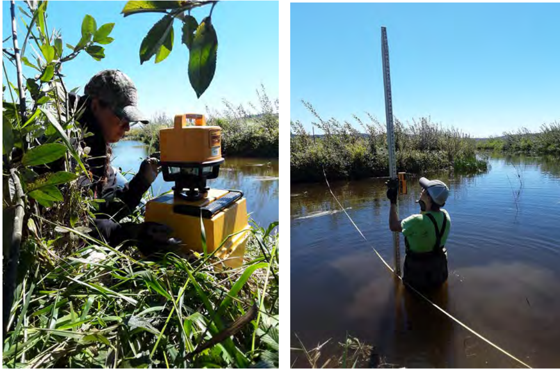
Figure 10. A laser level was used to complete some channel cross-sections in 2020 (left). If water depth allowed, 2020 channel cross-sections were completed on foot to maximize accuracy.
